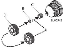
Eject with Ø 1.5 mm; 0.06 inch pin
