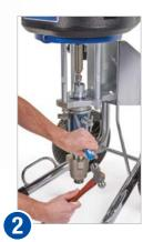
Loosen the jam nut
